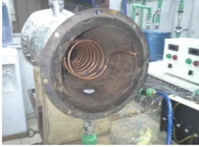
a) Photograph of the test section (shell and coil heat exchanger)
